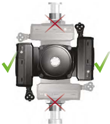
Position of Control Box
